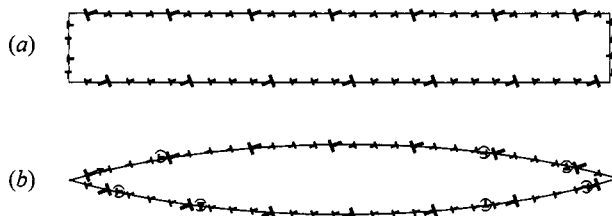
Figure 24.12: Formation of martensite inclusion. (a) Slab-shaped inclusion. Coherency dislocations present at ends that generate long-range stresses. (b) Lenticular inclusion. Coherency dislocations present at the ends in (a) are now distributed along the lens-shaped faces.
